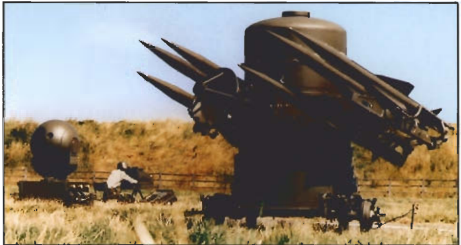
FIGURE 19 The Rapier uses Inductosyn transducers to transmit target tracking and missile launch angles.
